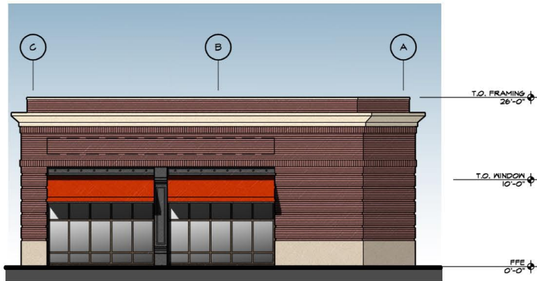
3 WEST ELEVATION A203 1/16" = 1'-0"
