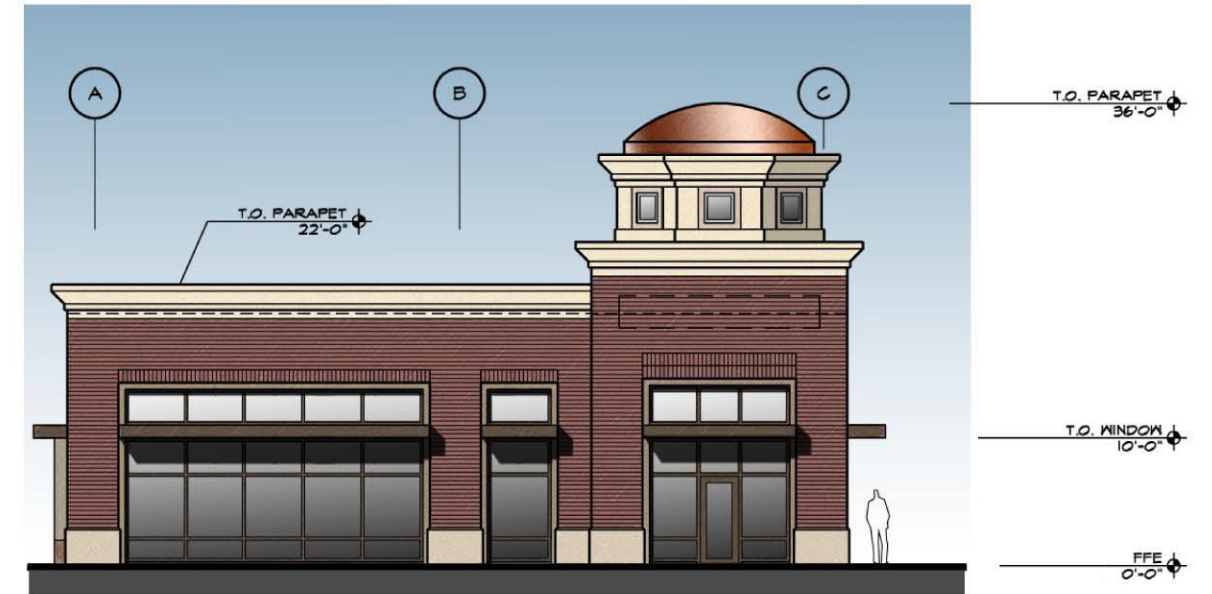
1 EAST ELEVATION A201 1/16" = 1'-0"
